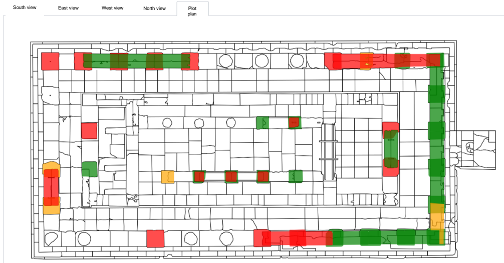
Figure 8. Coloring of structural members based on the most probable DS for the selected earthquake scenario.
