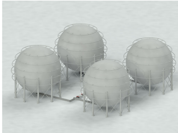
Fig. 1 Schematic illustration of typical spherical pressure vessels
