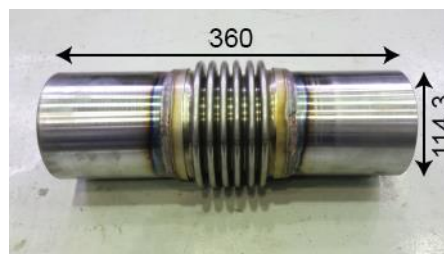
340 341 Figure 12: Flexible joint used in the experimental investigation
