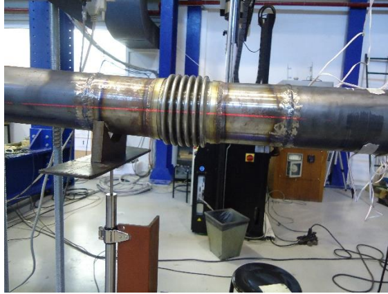
Figure 6: LVDT placed on a bellow's edge
