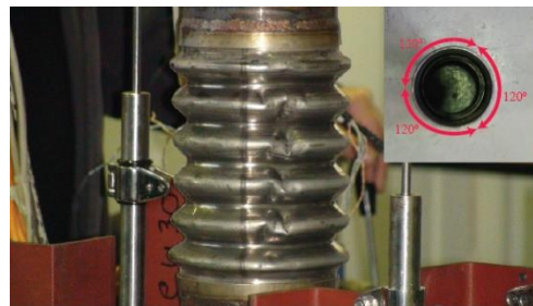
389 Figure 16: Joint failure in expansion through local deformations of the convolutions
